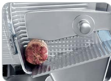
Design zavorra per piccoli salumi Fixing arm designed also for small sausages
